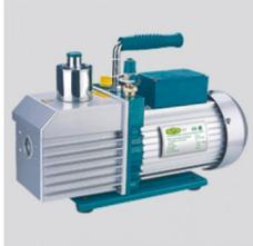
?????? ?????? REFCO ECO-9 Technical Data: Free air displacement: 9.0 cfm Number of stages: 2 Microns: 25 Intake threads: 1/4" and 3/8" SAE Flare Motor: 1 horsepower Voltage: 115 Volt, 60 Hz Power cord length: 78" Oil capacity: 2
